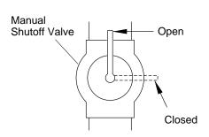
Figure 25 - Manual Shutoff Valve
